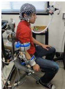
Upper-limb power-assist using EEG signals
